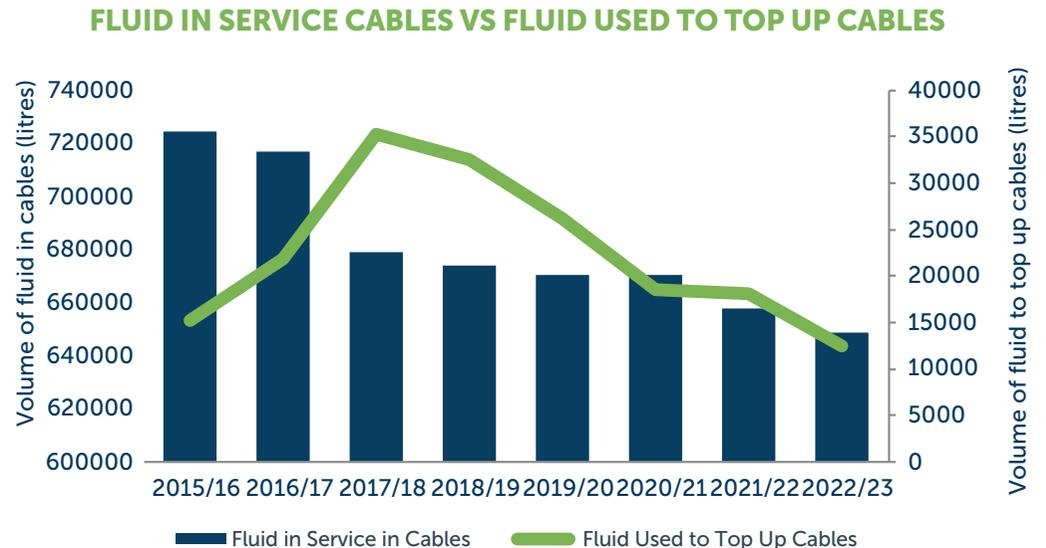
Figure 2: Oil in service cables vs fluid used to top up cables over the RIIO-ED1 period
