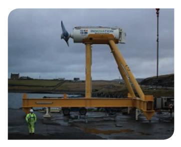
The picture above shows a tidal generator in the docks ready to be installed as part of the NiNES ANM scheme in Shetland.
