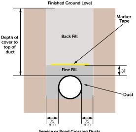
Service or Road Crossing Ducts (Note spare road crossing duct omitted for clarity)
