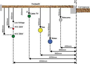
The cable depths referred to above apply to single cables and ducts. Where electricity cables and/ or ducts are installed above each other in the same trench please refer to our online technical guidance (TG-NET-CAB-001, Installation of Electricity Service, Intake and Distributor Cables up to and Including 33kV, available on our G81 library) for trench section details and separation distances.
