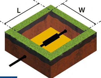
The length of the joint bay should be measured from the point where the new cable is parallel to and touching the existing cable for a breech joint. All cable joints should be in the centre of the joint bays.
