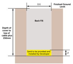
Trench Requirement for Mains Cables (SSEN to install cable, sand above the cable, sand to be provided by developer, and apply marker tape. Developer to complete back fill)
