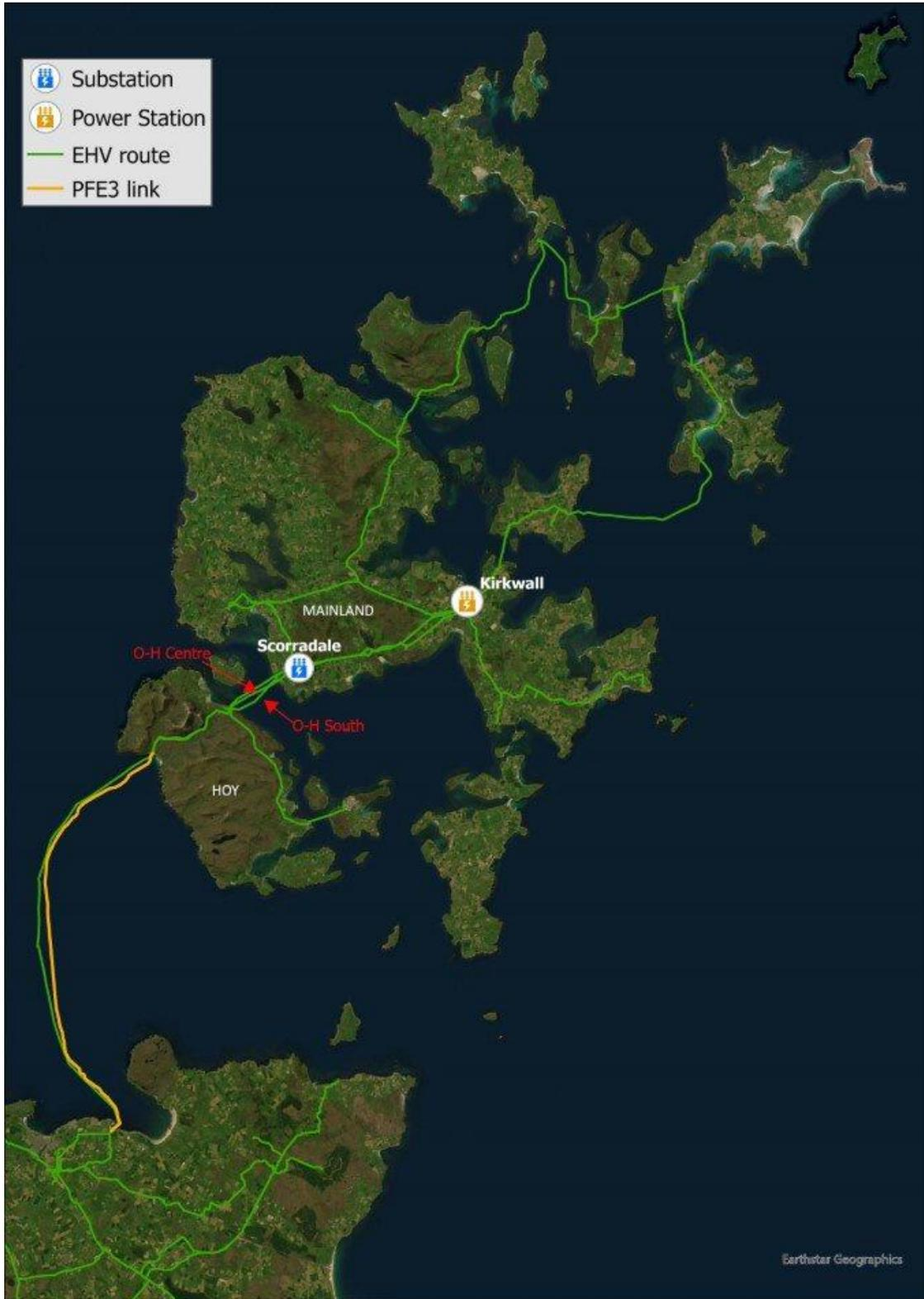
Figure 3: Existing 33kV network supplying Orkney
