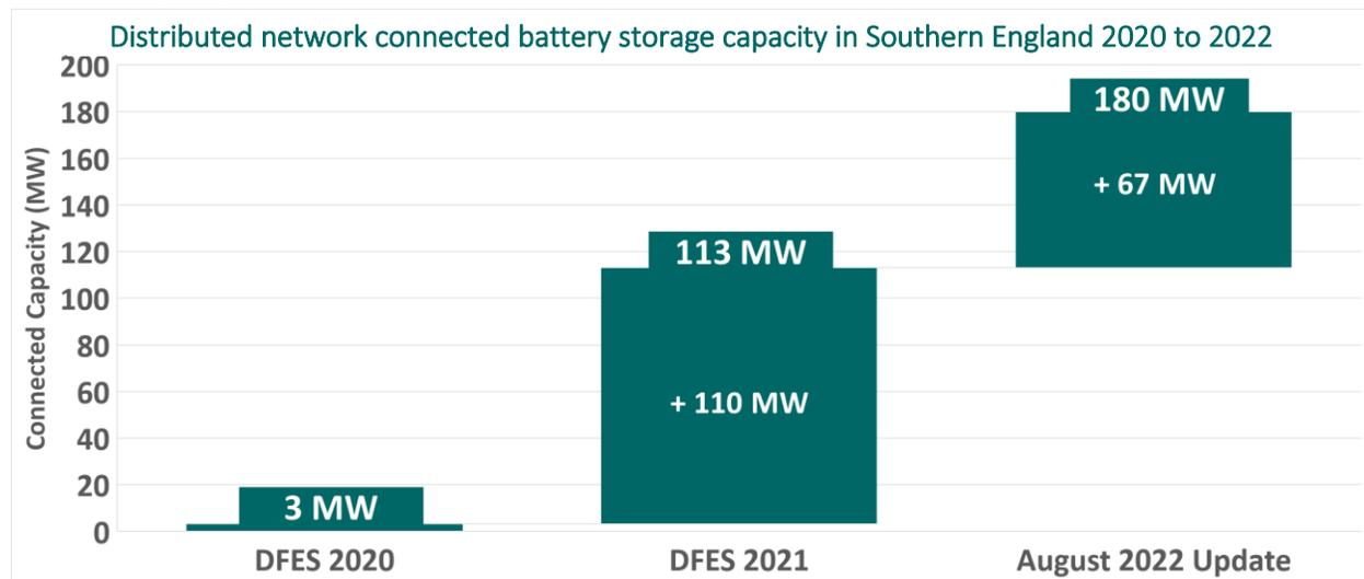
Figure 12: Battery storage capacity connected to the distribution network in Southern England (2020 to Aug 2022)
