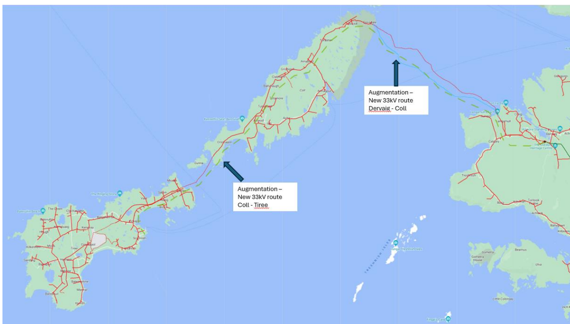
Figure 26 Network schematic with system needs 2041-2050 Option 2 – 33kV on Existing Route
