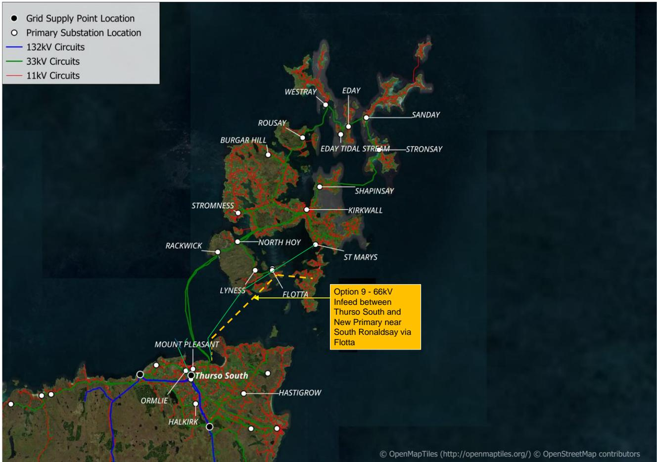
Figure 37 Network schematic with system needs 2041-2050 Option 9.
