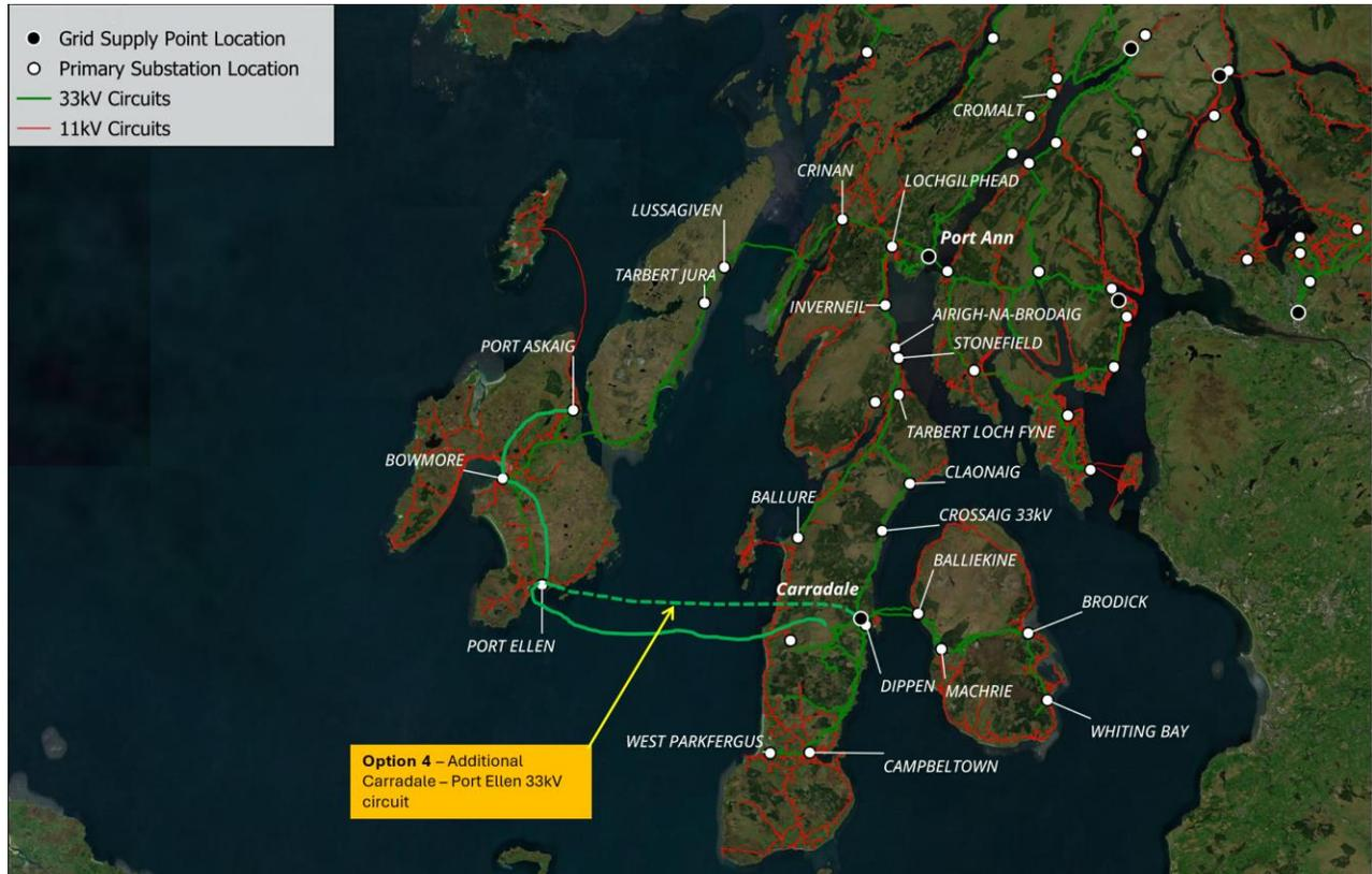
Figure 33 GIS view of network with works in progress and additional reinforcement options by 2040 (Option 4)
